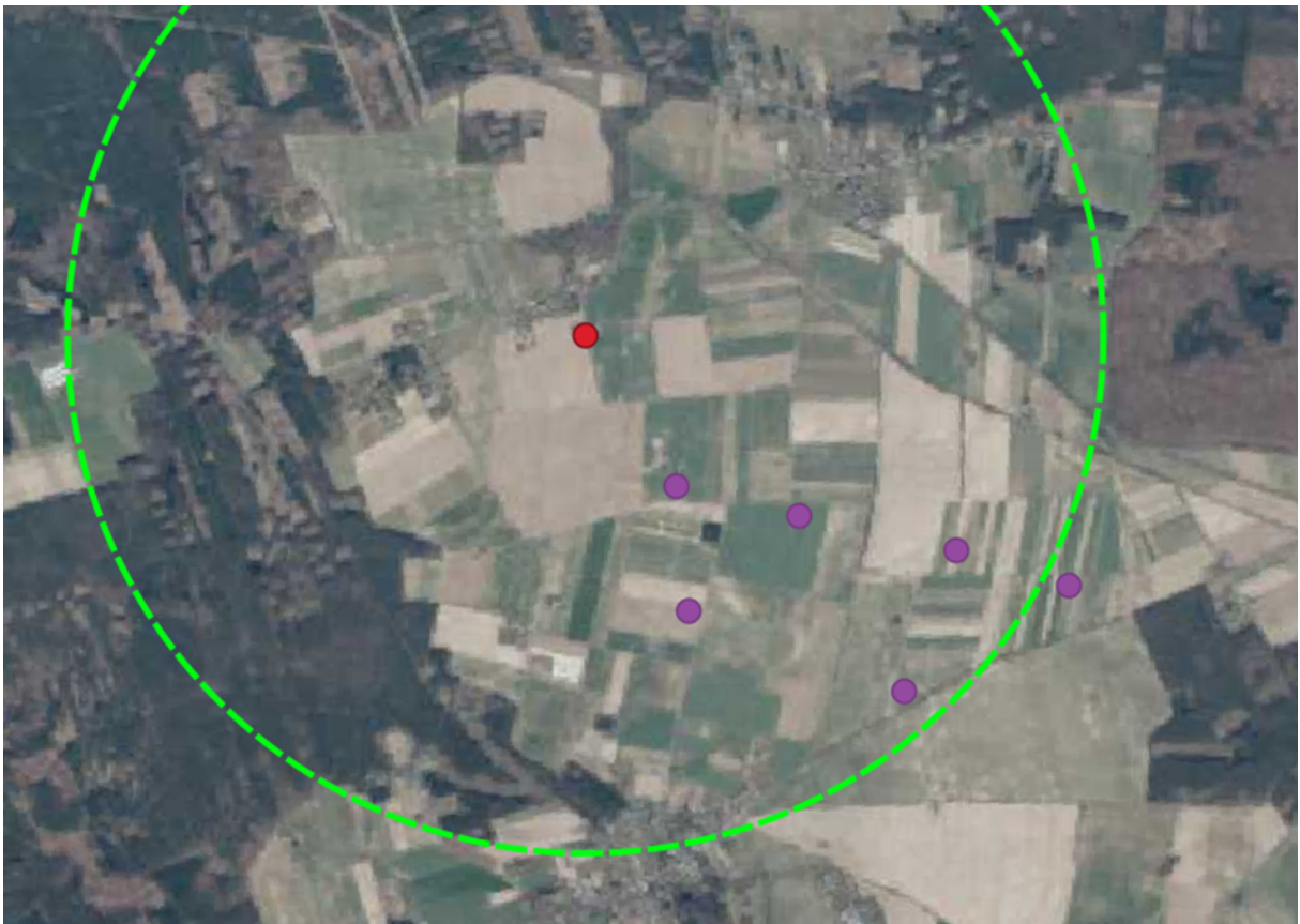
Figure 9. Wind turbines location (purple points) and measurement point (red point) – turbines inside green circle should be off during background noise measurements.
