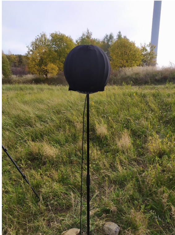
Figure 41. An alternative set of double wind shield for measuring wind turbine infrasound noise.
