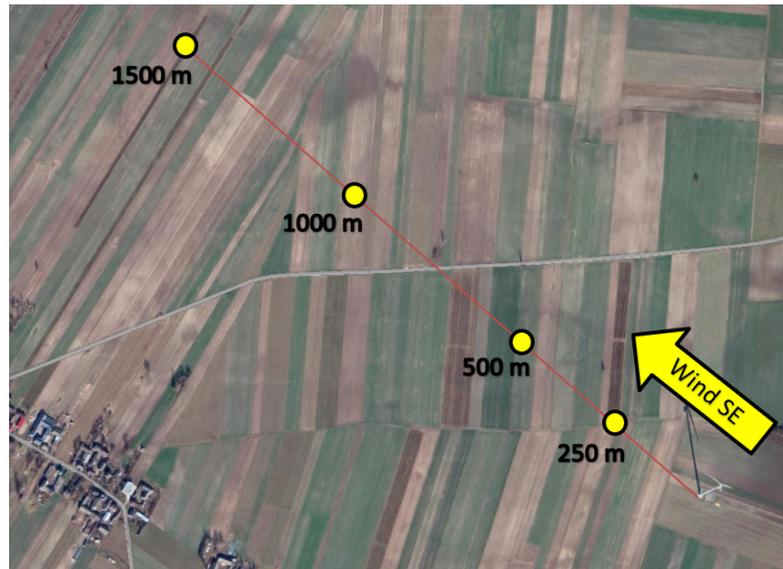
**Figure 1.** Distribution of measurement points in relation to the wind turbine
